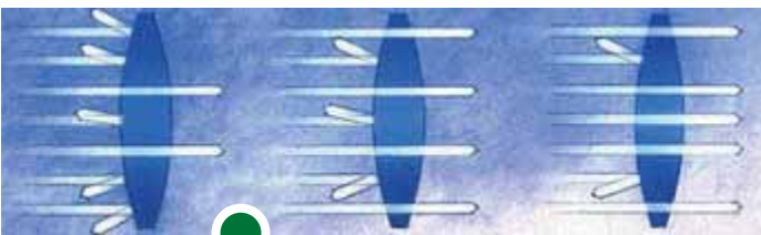
Light transmission is influenced by lens quality and coating.
